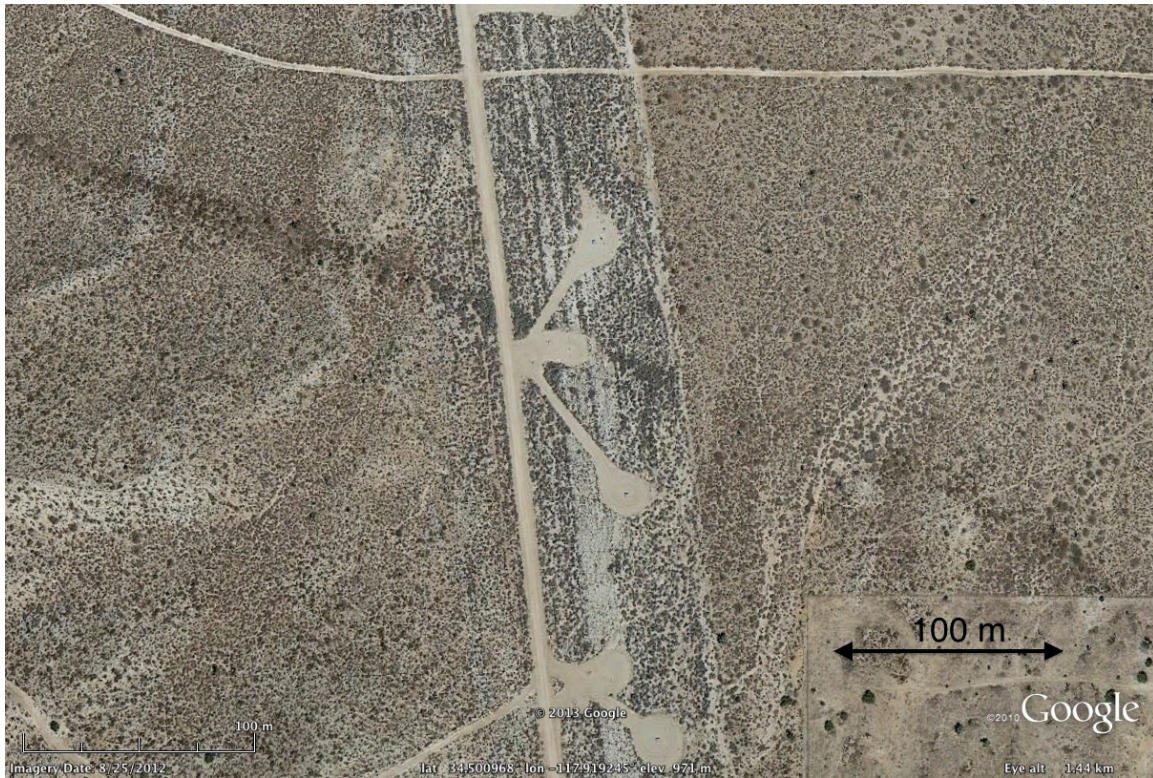
Figure 3 Google Earth image of an underground section of the California Aqueduct crossing VL2. The ground was scraped clean during construction and VL2 has reestablished itself in the disturbed soil. At the left are twin chevron-shaped outcrops uphill (toward the bottom of the picture) of VL2. Field investigations found them to be fine-grained granitic rock. The apices of the chevrons are parallel to the VL. The northern terminations of the outcrops coincide with the VL. North of the VL, no outcrops are present, and only eroded and deposited grus is found.
